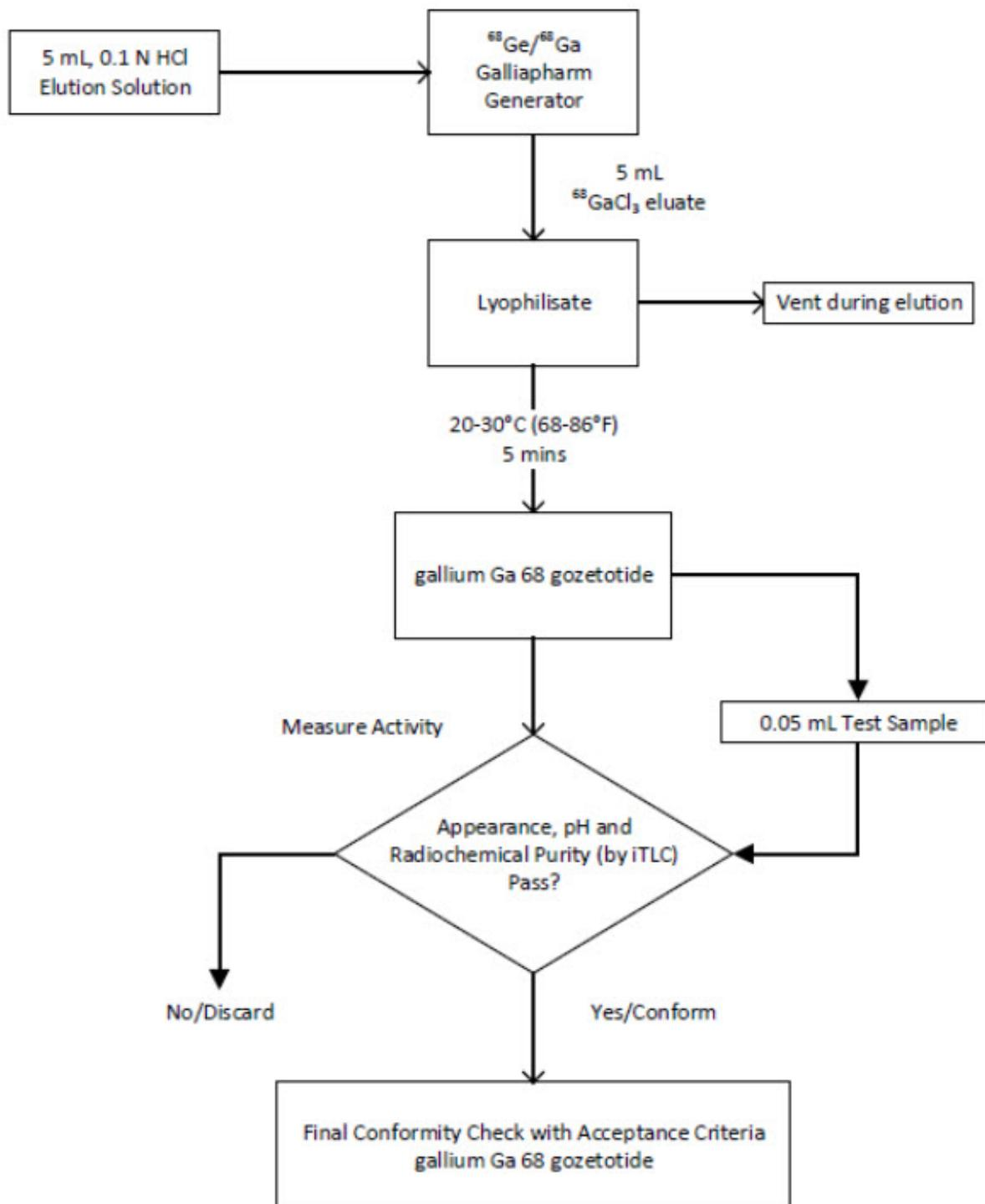
**Figure 2. Preparation with IRE ELiT Galli Eo Generator**
